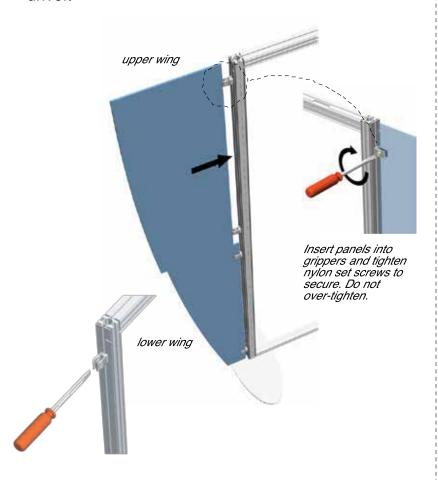
Connect 4 panel grippers to upper vertical extrusion (nylon set screw facing back) and tighten. Insert header into grippers and tighten nylon set screws to secure. Do not over-tighten.
