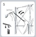
To attach light fixtures, first disengage the upper channel bar from the top hub and tilt downward. Push the light fixture down into the top of the channel bar. Tilt channel bar with light fixture back up and re-engage to the top hub. Drape cable over the frame.
