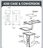
Case Assembly: Place the frame case and the panel case . Align upper two and lawer two latches and Latch together.
