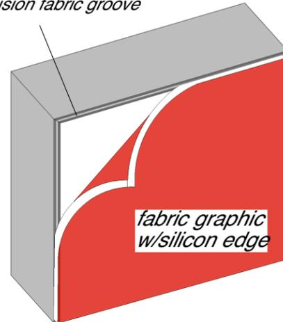
Insert the silicon edge of the fabric into the groove of the extrusions.
