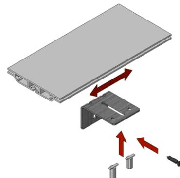
Attach wall bracket to top extrusion groove with provided hammerhead screws. Locate position of wall bracket on extrusion (preferably by wood stud) by sliding the bracket on the extrusion and tighten it. Secure the frame to the wall with provided wood screw.
