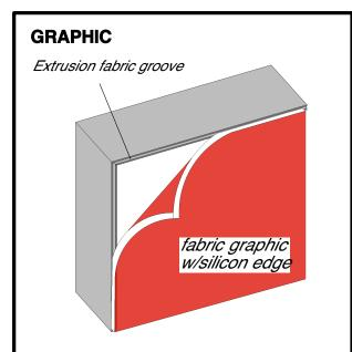
Insert the silicon edge of the fabric into the groove of the extrusions.
