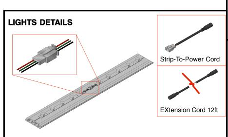
Lights come attached to extrusions. Ensure all lighting strips are connected. Once frame is assembled, connect strip-to-power cords to the end of top and bottom lights chain.
