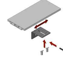
Attach wall bracket to top extrusion groove with provided hammerhead screws. Locate position of wall bracket on extrusion (preferably by wood stud) by sliding the bracket on the extrusion and tighten it. Secure the frame to the wall with provided wood screw.
