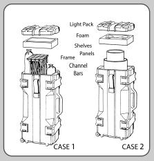
**Case packing:** Collapse frame, pack in box and insert into Case1. Pack lights & channel bars in bags and pack in Case1. Roll up panels fabric to fabric and insert into Case2, Cases can be strapped together to roll as a complete unit. **Note:** Graphics Roll Individually with image side out against a plastic liner.
