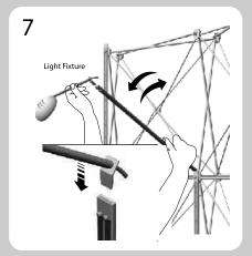
To attach light fixtures, first disengage the upper channel bar from the top hub and tilt downward. Push the light fixture down into the top of the channel bar. Tilt channel bar with light fixture back up and re-engage to the top hub. Drape cable over the frame.
