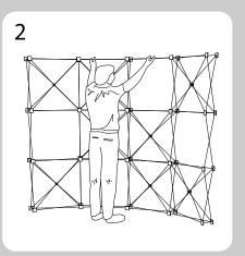
Frame should pop into a fully open and upright position. Yellow dots on bottom row of hubs should be on the floor.
