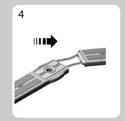
Connect each three-section channel bar assembly by inserting the sections that are pre-attached with bungie cords. By straightening out the channel bar assembly the bungie cords will automatically align the assembly.
