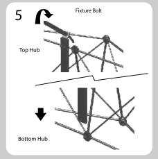
Place the channel bar assembly onto the frame by first attaching it to the top hub. Slide it onto the top hub, then slide the Lower channel bar onto the bottom hub. Slide gently downward to engage.
