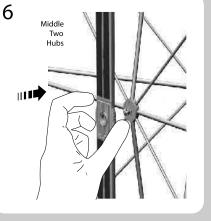
Attach the center sections of the channel bar assembly to the middle two hubs by pushing the channel bar assembly onto the hub. The bushing on the hub should engage through the hole in the connector assembly. Repeat for remaining channel bars at all panel locations.
