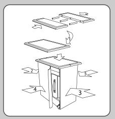
**Case Conversion:** Assemble top as shown and place on cases. Attach panels in numbered order shown. Velcro blotter to table top.
