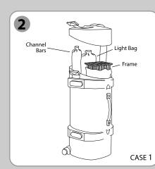
Collapse frame, pack in bag and insert into Case 1. Pack lights in bag and pack in Case 1 next to channel bar bag as shown.
