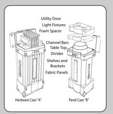
**Case packing:** Collapse frame, pack in box and insert into Case A. Pack shelves & channel bars in bags and pack in Case A. Roll up panels fabric to fabric and insert into Case B. Cases latch together two places to roll as a complete unit. **Note:** Graphics Roll Individually with image side out against a plastic liner.
