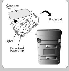
Pull back the foam cover inside the main lid to insert the lights, extension cord and power strip. Replace foam and insert the conversion top, or plastic shipping protector. Attach velcro straps to hold in place. Flip over Lid and close all 4 latches.
