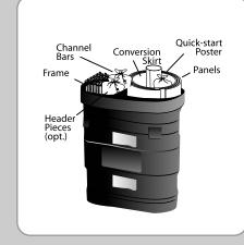
**To pack:** Roll up panels in pairs, surface to surface, and insert into the round side of the case. Place frame & channel bars into bags, insert into other side of case.
