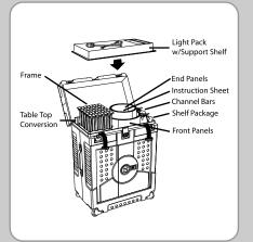
**Case Packing:** Roll and load skirts followed by panels and ends. Load your frame next followed by the channel bars, shelves, headers and table top conversion. Connect support straps and lay the light pack on top of straps. Close lid and lock. Refer to inside of case lid for additional instructions.
