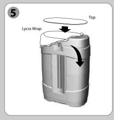
**Case Conversion:** Stretch the Lycra skirt over the empty case as shown with the seam of the skirt at the rear of the case (wheel side).
