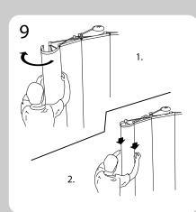
1. Lift end panel and guide front notch of plastic plate over front peg. Hook the other side on the panel peg at the back of the frame. 2. Slowly run your hands down the sides of the
