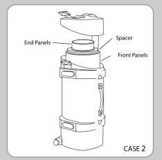
Roll up panels fabric to fabric and insert into Case 2 as shown. Once two cases are loaded they can be strapped together for easy transport.
