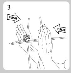
Ensure that spacer bars are fully engaged and locked.
