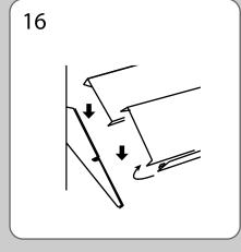
Snap the literature strip onto the front edge of the shelf after shelves are installed.
