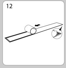
Place the assembled frame on the floor with the velcro side facing up. Roll up the graphic panel, making sure the velcro is on the outside. Matching the end of the graphic to the end of the frame, slowly unroll the graphic while guiding your hand along the edge to keep it even. Press to secure.
