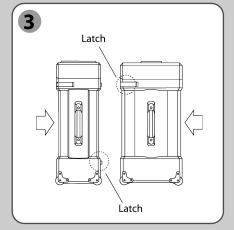
**Case Assembly:** Place the frame case and the panel case next to each other with handles on same side. Align the upper two and lawer two latches and Latch together.
