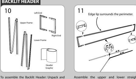
Assemble the upper and lower straight sections by inserting A side (with metal spring) into B side, as shown in detail illustration above. Insert the U-shaped end pieces into the ends of the assembled straight sections.
