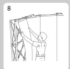
Hold a front panel on its side edges about 1/3 of the way down from the top. Lift section and guide notches over the panel pegs on the top hubs. Slowly release the panel, allowing it to roll down the channel bars. Repeat for all front panels aligning them as you go.
