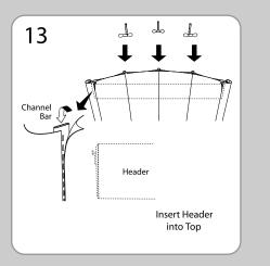
Lift the completed header assembly and hang it by inserting the brackets into the top of the channel bars. Hang lights by inserting the light bracket into the top of the channel bars.
