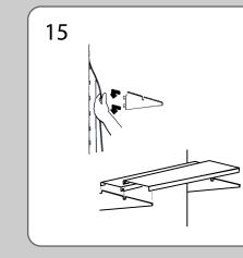
Insert bracket tabs into the slots and push down into place. Place the second bracket level with the first. Attach each shelf with the notches facing the back. Secure each shelf by making sure it is pressed down into the slots in the brackets.
