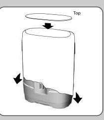
Pull down to conceal the case. Place the counter top onto the top attaching it to the Velcro.
