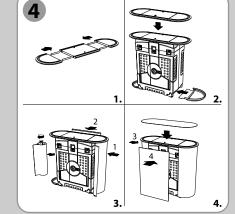
**Case Conversion:** Assemble top and secure to case using a coin to tighten the two fasteners. Slip an end tray under both sets of wheels. Store panel liners and bags under table top overhang. Attach panels in numbered order as shown.
