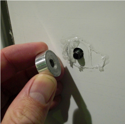
Place sintra onto the studs in the grooves of the M1020. Secure in place with 3/4" polished standoff caps.
