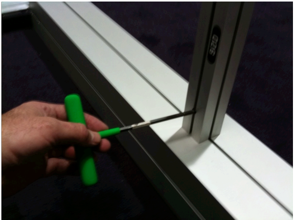
Use the green tool provided to secure the #041 and #042 to the octanorm #038 and #039
